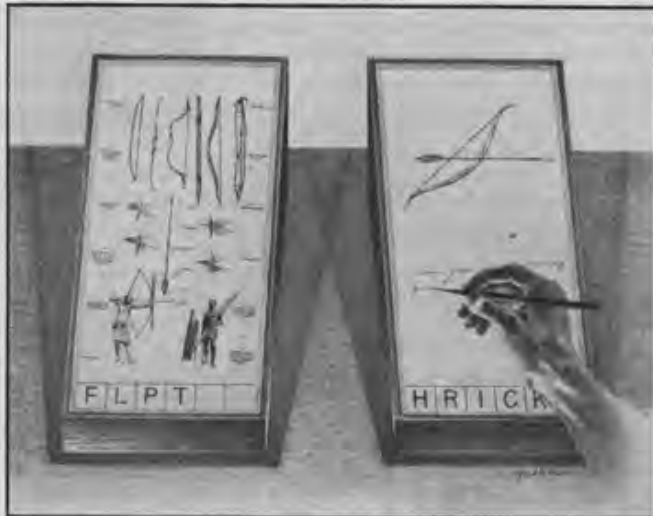
MEMEX IN USE is shown here. On one transparent screen the operator of the future writes notes and commentary dealing with reference material which is projected on the screen at left. Insertion of the proper code symbols at the bottom of right-hand screen will tie the new item to the earlier one after notes are photographed on supermicrofilm.
